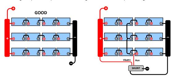
In an unmonitored battery bank the midpoints should not be interconnected, one bad battery bank can go unnoticed and could damage all other batteries.
