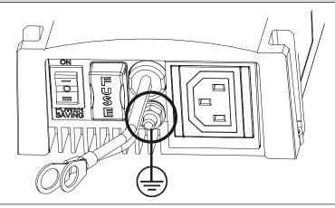
Step 7. Connect the battery to the DC input. Do not place the fuse yet!
