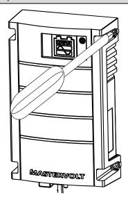
Step 6. Connect the chassis ground terminal to the central grounding point of the vehicle/ship.
