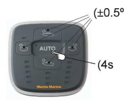
In the automatic mode, press any of the four buttons to alter the setting 0.5 degrees in a certain direction. Press more times for a greater change.
