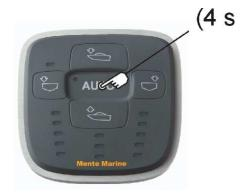
Run the boat at cruising speed. Manually control the trim tabs until you find the best attitude. Then, press and hold the auto button for 4 s, until the AUTO indicator is lit up.
