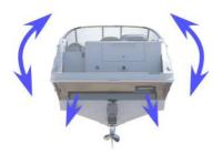
ACS AD automatically adjusts the boat to the optimum attitude in the pitch axis, improving visibility and also enabling speeds in the "semi-planing" range. It also improves the "hole shot".
